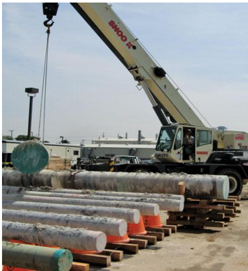
Sections of pipe are removed at GTI’s field-applied pipeline coatings testing site.
